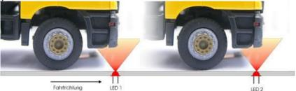
By passing the first LED the car decelerates and at the second it stops. On vehicles increased stopping distances multiple LEDs can be desirable. Each LED has its own series resistor connected to the corresponding output.
